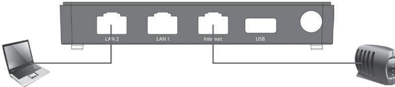
*Figure 2 Connecting Kerio Control Box NG100 to the network*
